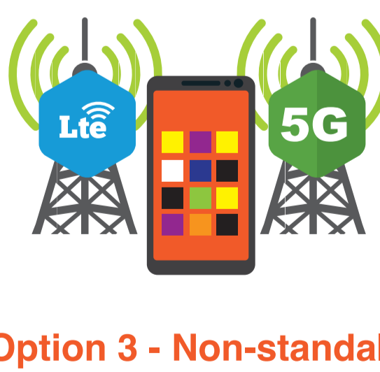
Option 3 - Non-standalone (NSA) or EN-DC (E-Ultra New Radio Dual Connectivity)
